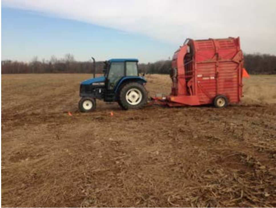
Figure 1. Stover being removed with Hess hay stacker.
